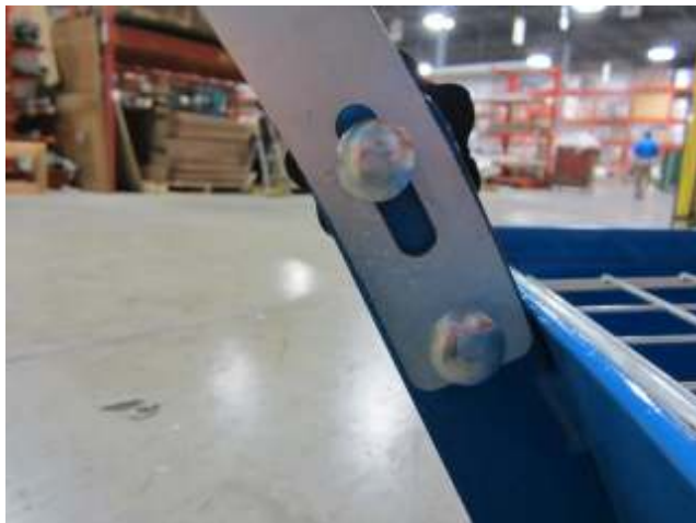
Step 6: Slide slot onto the stud
