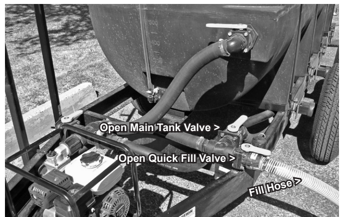
Figure B29 Filling Through Quick Fill (1,025 Gal.)
