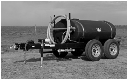
500 Gal. Fire Control Trailer
