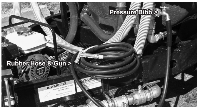
Figure B38 Rubber Hose on Pressure Bibb
