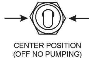
Figure 38. Pumping Control Switch Center Position (No Pumping)
