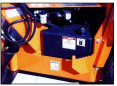
No more fuel sight gauges and hard to clean fuel tanks. The polyethylene fuel tank eliminates rust contamination and is easily removable should fuel become contaminated. The fuel tank features a top mounted mechanical gauge for quick, easy fuel checks.
