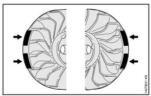
The new ignition systems used on some models can be identified by their flywheels with **two** pairs of magnetic poles.
