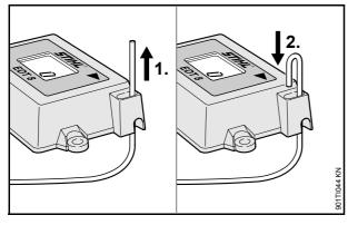
Both the test line and the antenna can be attached to the housing in the same simple way, as illustrated above.
