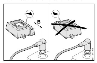
This method is useful if a test line cannot be used and when the measurement must be made close to the engine or to the pulse-conducting parts of the ignition system.
