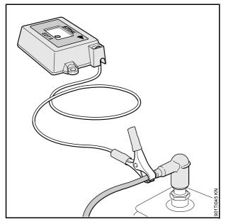
Pulses should be measured with the test line. This method yields the most accurate results.
