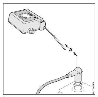
This method is useful for measuring the speed of engines in which it is difficult or impossible to clamp the test line onto the ignition lead or spark plug boot.
