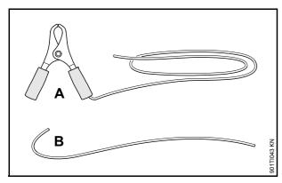
The two new tachometers are supplied complete with two antennas of different lengths:
