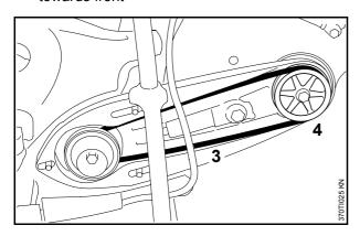
• Remove the V-belt (3) from the front pulley (4)
