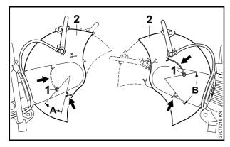
In STIHL Cutquik® TS 410, 420 cut-off machines, the adjustment range (**A** and **B** respectively) of the guard will be determined by the stop pin (**1**) installed into the cast arm and by the lugs (arrows) molded onto the guard (**2**).
