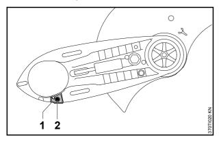
With the introduction of the new guards (see  $\square$  1.3), the limit stop (1) 4238 691 0200 and the stop pin (see  $\square$  1.4) are introduced. The limit stop (1) is fastened to the cast arm with the pan head self-tapping screw IS-P4x16 (2) (9074 478 3025).
