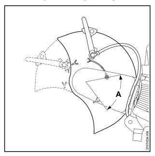
Rotate the guard forwards and backwards as far as possible – adjustment range (A) must be limited by the stop pin
