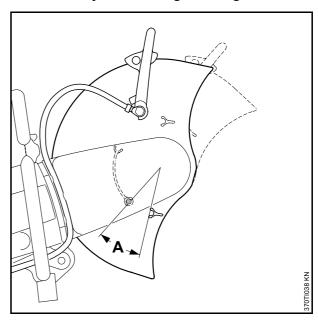
Rotate the guard forwards and backwards as far as possible – adjustment range  $(\mathbf{A})$  must be limited by the stop pin
