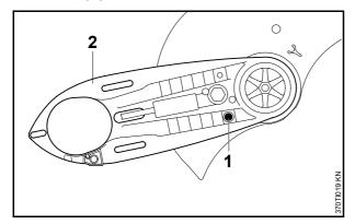
With the introduction of the new guards (see (1.3), the stop pin (1) 4224 691 0100 and the limit stop (see (1.5) are introduced. The stop pin (1) installed into the cast arm (2), together with the lugs molded onto the guard (see (1.3)) determine the adjustment range (see (1.1)).
