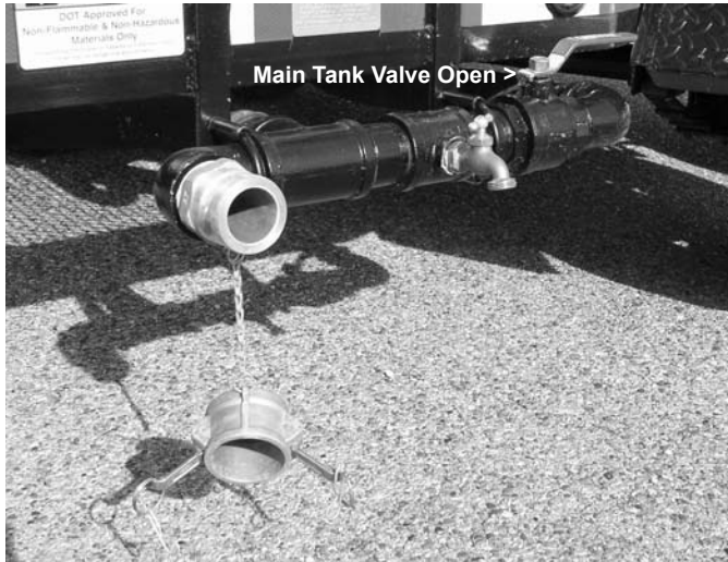
Figure C1 Main Tank Drain
