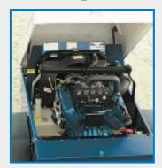
The hoods are equipped with gas-assisted lift cylinders providing easy access for inspection, cleaning of coolers and servicing.
