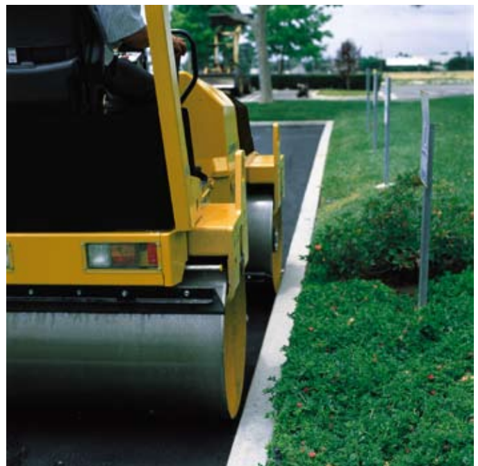
Offset drums allow close operation against walls and curbs and increase the working width of the machine.
