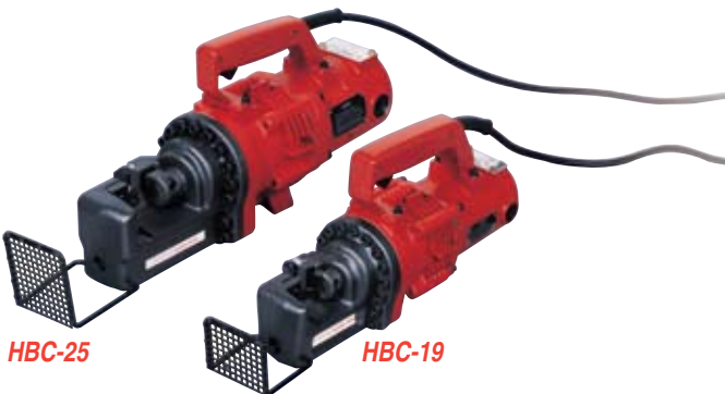
HBC-series models are available with cutting capacities up to 1" in diameter. Each cutter is powered by a miniature hydraulic pump and 115-volt electric motor.
